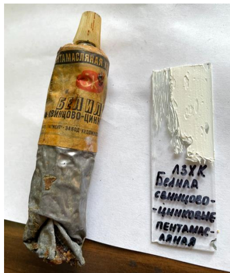
Fig. 10. Model specimen of penta-oil paint (spectrum and position on the TIC chromatogram).
